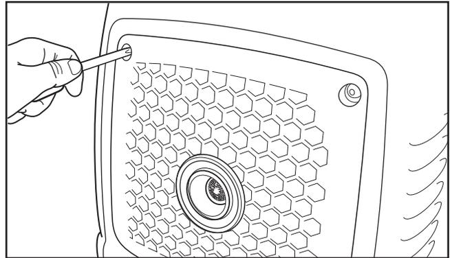
2. Remove screw that attaches spark arrester screen to muffler. Remove spark arrester screen.
