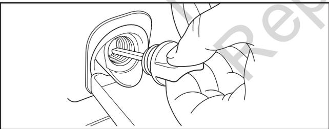
4. Using oil funnel (optional), slowly pour contents of provided oil bottle into oil fill opening to the point of overflowing at oil fill cap.
