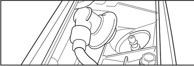
4. Remove spark plug and inspect spark plug.
