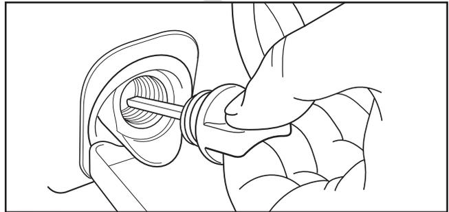
5. Replace and tighten oil fill cap.
