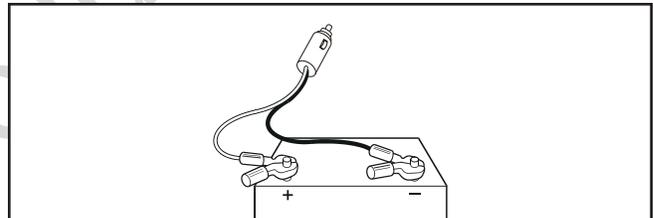
6. Connect battery charge cable clamp with **black** handle to battery post or terminal indicated by **Negative, NEG**, or (-).
