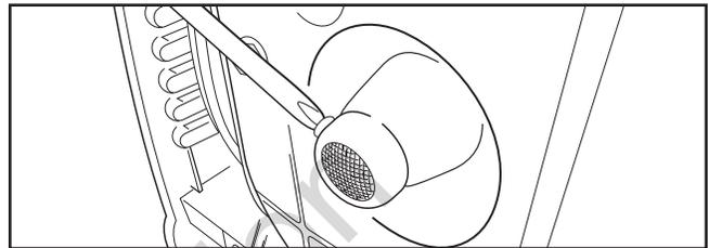
3. Inspect screen and obtain a replacement if torn, perforated or otherwise damaged. DO NOT use a defective screen. If screen is not damaged, clean it with a brush.
