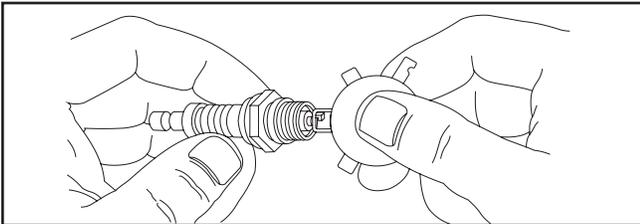
7. Install spark plug and tighten firmly. Reinstall spark plug boot.
