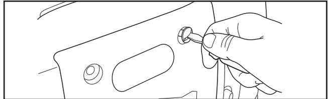
3. Clean area around oil fill and remove oil fill cap.
