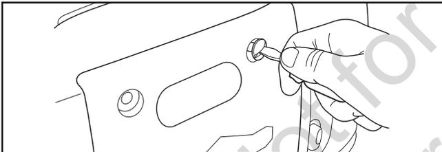
3. Clean area around oil fill and remove yellow oil fill cap.
