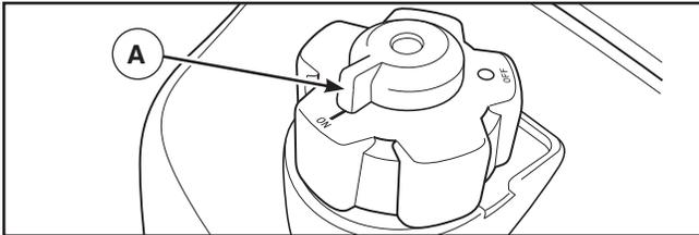
When the engine is not in use, leave the vent lever in the OFF (0) position to reduce the possibility of fuel leakage. Allow the engine to cool before turning the vent lever to the OFF (0) position.
